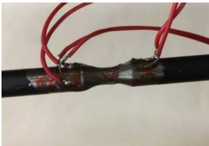
Fig. 4 – Representation of the installed strain gauge
